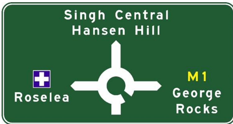
Figure 6.5(a) – Standard advance roundabout direction sign
