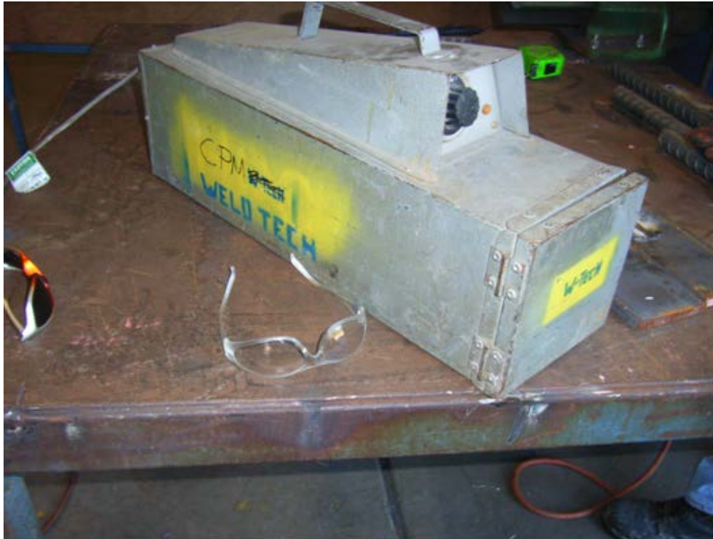
Figure 2 – Incorrectly stored hydrogen controlled electrodes
