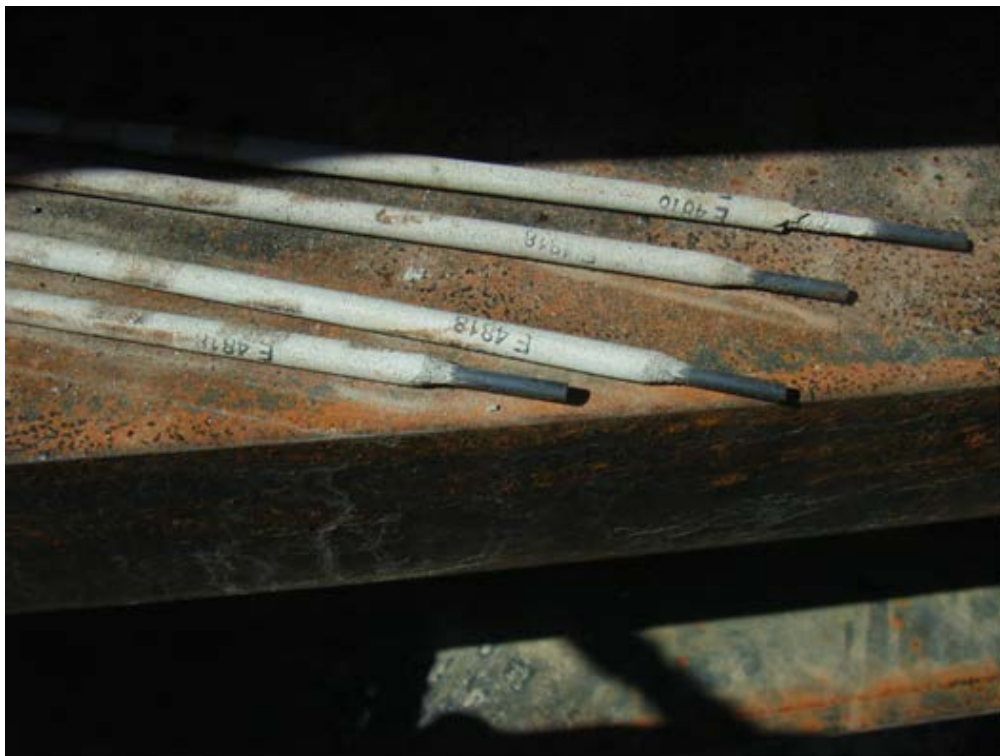
Figure 2 – Incorrectly stored hydrogen controlled electrodes
