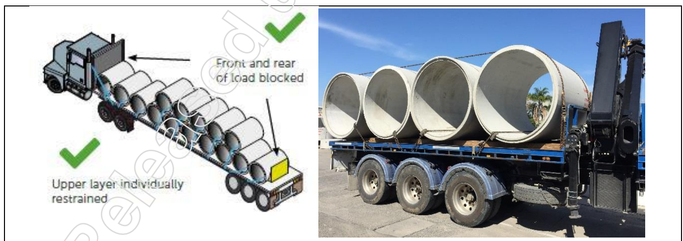
Figure 1: Transverse loading example
