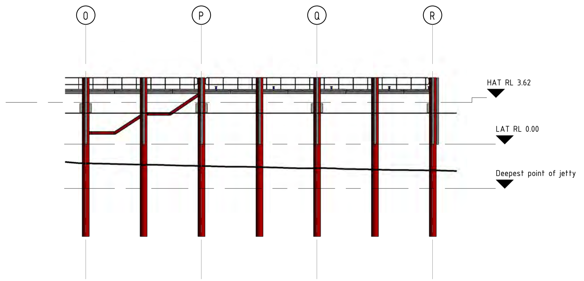
FENDER PILE ELEVATION 1: 200
