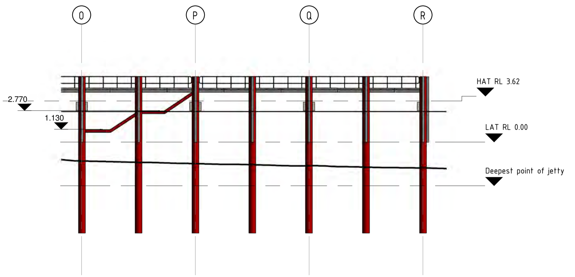
FENDER PILE ELEVATION 1: 200
